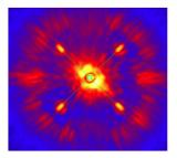
In SPHERE's pupil-stabilized mode, the field rotates !  $\rightarrow$  exact position of the rotation center is critical for astrometric measurements
