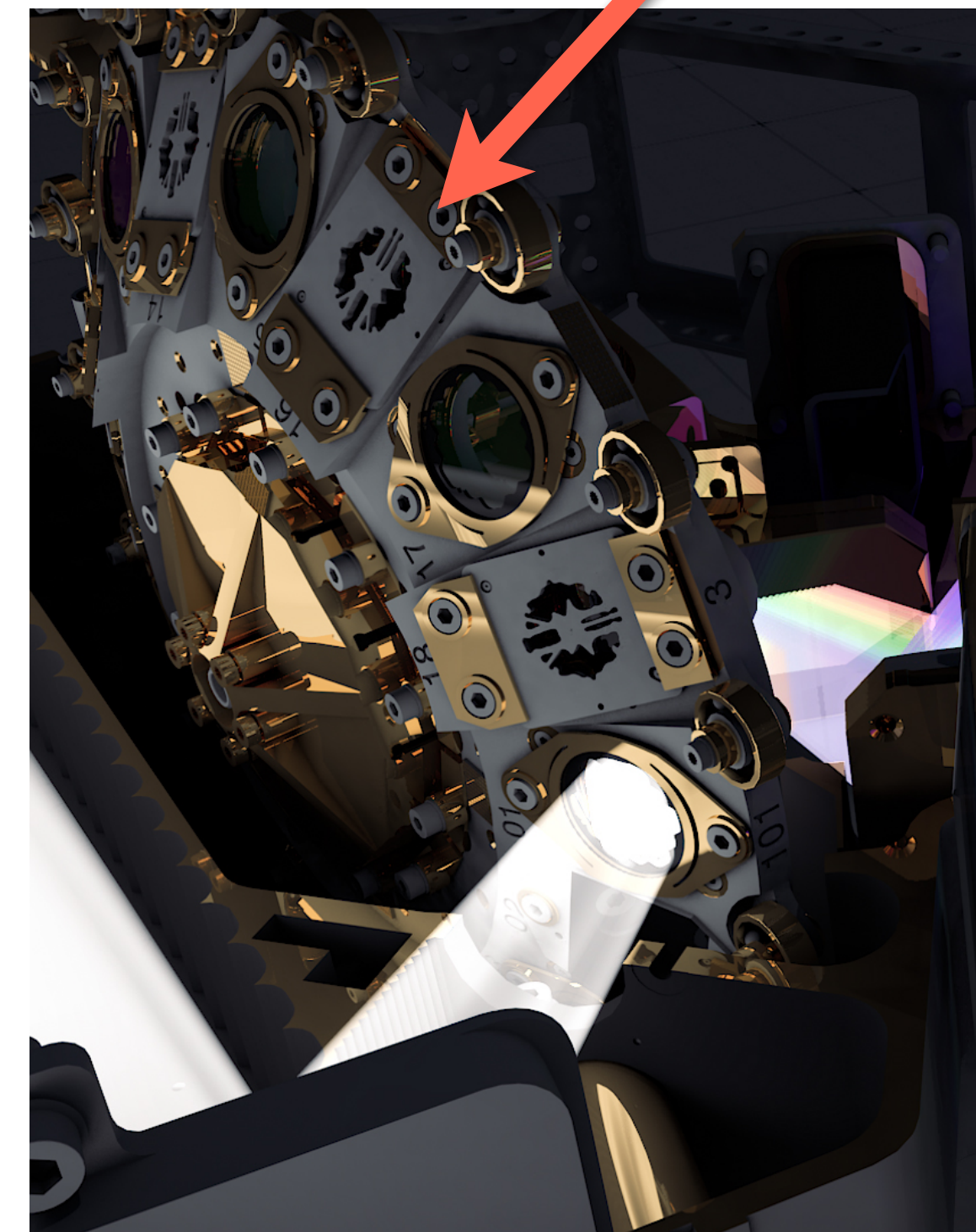
2. Lyot stops+IR filters in the filter wheel
